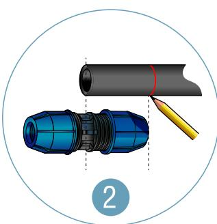
Mark the insertion depth on the pipe according to the "Insertion Table".
