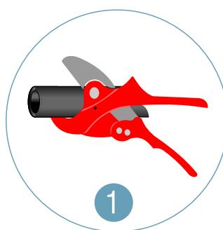
Cut the pipe with a proper pipe cutter. Clean the burr at the pipe end.
