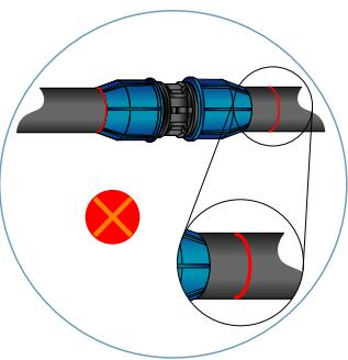
The pipe is not fully inserted into the fitting.
