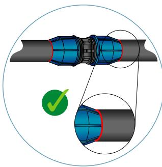
Ensure the marking on the pipe is as shown in the picture. To ensure the fitting is fully fastened, ascertain that the locking nut exceeds the last thread of the body.
