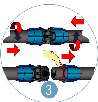
Loosen the locking nut by 2 or 3 threads without removing the locking nut, insert pipe into the fitting to the correct depth according to the "Insertion Table".
