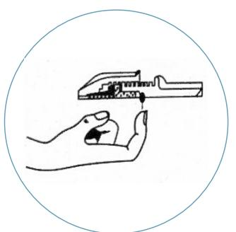
\*Size: 40, 50, 63, 75, 90 & 110mm. The NBR O-ring should be adjusted back to the correct position with your finger before pipe is being pushed in and tightened.
