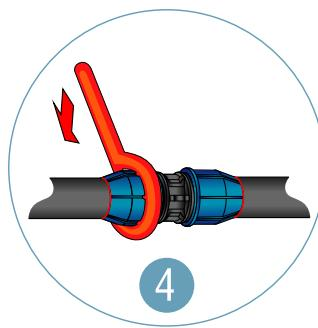
The locking nut can be tightly fastened by hand up to size 32mm OD. For sizes larger than 32mm OD, it is advisable to use strap wrench or other proper tools.
